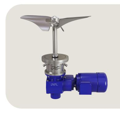
The shaft rotates, turning the EnSaFoil impellers. The impeller movement creates a high flow with low shear due to the highly effective axial pumping effect on the liquid in the tank. This results in effective mixing and blending of the entire contents of the tank.
